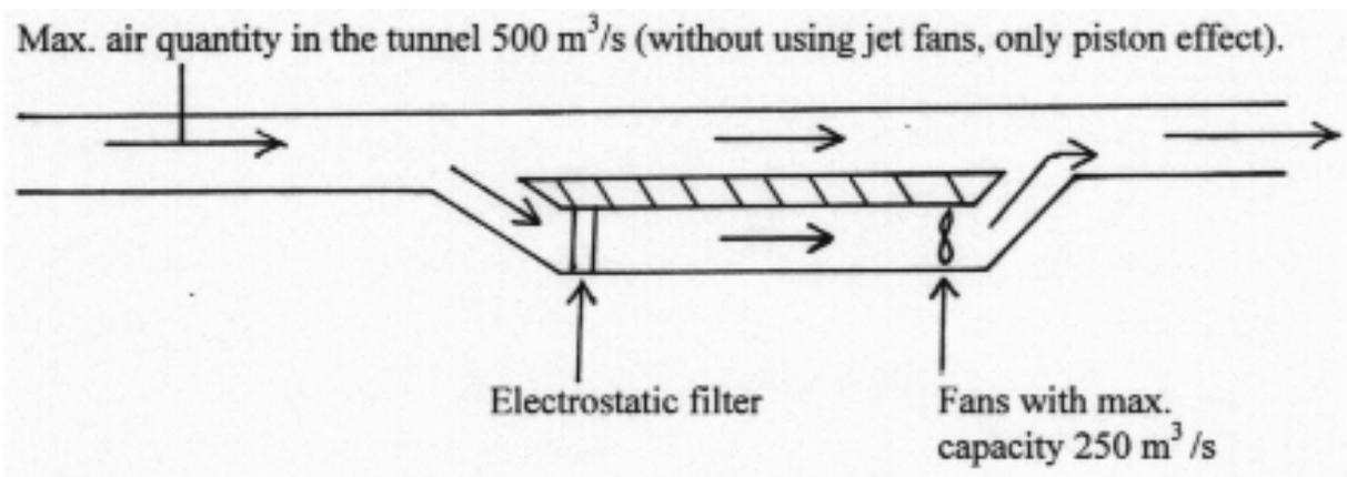
Fig. 5 A principle draft with air flows and air quantities in the tunnel and the cleaning bypass.
