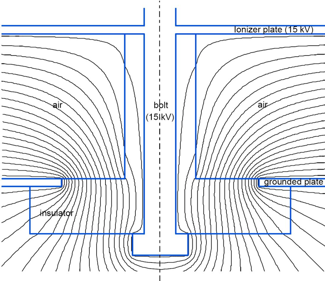
Fig. 2: Equipotential lines of the electric field in the surrounding of the insulator for the ionizer
