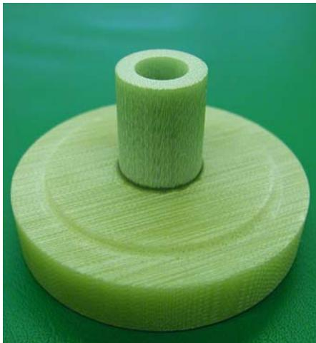
Fig. 1a: Detailed view of the insulator
